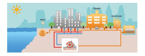
The technology is based on heat pumps boosting the temperatures to desired levels:
